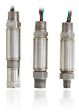
**Environmental Data** Temperature Operating Ambient -40 to 85°C (-40 to 185°F) Operating Media -55 to 125°C (-65 to 250°F) Storage -55 to 105°C (-67 to 221°F) Thermal Limits Compensated Range -20 to 70°C (-4 to 158°F) TC Zero: <±0.5% FS TC Span: <±0.5% FS Other Shock EN 60068-2-27 Vibration EN 60068-2-6, 60068-2-64, and IEC 68-2-32 EMI/RFI Protection: Rating: IP-65 (vented), IP-66(factory sealed)
